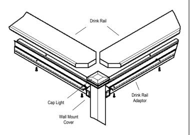
**c. Crossover:** Take 2 drink rail adaptors and cut 3/16" off inside corners of each adaptor at 45-degree angle. Measure distance between crossover connectors. Mark drink rail adaptor end away from corner for overall length and cut adaptor accordingly.
