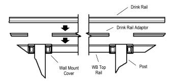
b. Wall Mount with Cap Light or Flat Cap: When a cap light or flat cap is used post will need to extend 21/4" above top of wall mount cover to prevent interference with drink rail. A longer post will need to be ordered to accommodate this. Measure distance between wall mount covers and cut drink rail adaptor accordingly.
