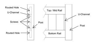
Tri-Max II: Put on top rail locking it in both posts. If installing 7' or 8' tall section, insert mid rail (with aluminum reinforcement) into post with the preformed opening faced up and the routed opening faced down. Repeat above procedure.
