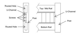
Screw U-Channel to post (screws provided), spacing screws evenly. Insert bottom rail (with aluminum reinforcement) into post. Let the rail go in until you can get the opposite end of the rail into the opposite post and lock it in. Insert vertical panels into bottom rail.
