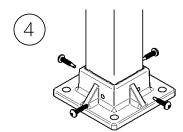
Insert (4) 12x1" self-tapping screws, into holes in mount. Use drill with #2 square drive bit.
