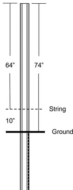
Sections installed on Standard Post will typically have 2" ground clearance.
