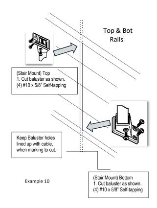
Please note: Begin by inserting screws into the top mount first. Then, Plumb the baluster and insert screws accordingly. Level mount screw holes should be facing inside toward stairs for ease of installing screws.
