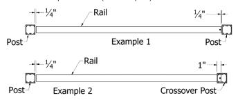
Crossover Railing: Cut bottom rail the same as (Example 1). For top rail, make end spacing exactly 1" longer on all ends connecting to line crossover post (Example 2). If connecting to a corner crossover cut top rail 1/4" short of post.
