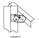
When installing bottom rail, lay (with approximately 1" clearance from the nose of the steps) beside the posts. Clamp rails to post. Hold swivel stair mounts up against posts and beside the rail to determine where rails are to be cut to fit inside the swivel stair mounts. Mark posts for each stair swivel mount position (Example 6).
