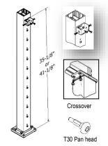
**NOTE:** If screw stops penetrating rails, rotate screw in reverse several revolutions while maintaining penetration pressure to remove potential material burr from tip of screw. Then continue to install screw, repeat, as necessary.
