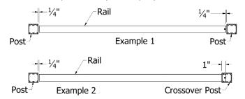
Crossover Railing: For top rail, make end spacing exactly 1" longer on all ends connecting to line crossover post (Example 2). If connecting to a corner crossover cut top rail '4" short of post.
