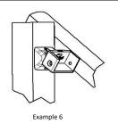
Clamp rails to post. Hold swivel stair mounts up against posts and beside the rail to determine where rails are to be cut to fit inside the swivel stair mounts. Mark posts for each stair swivel mount position (Example 6).
