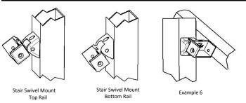
2. Clamp rails to post. Hold swivel stair mounts up against posts and beside the rail to determine where rails are to be cut to fit inside the swivel stair mounts. Mark posts for each stair swivel mount position (Example 6).
