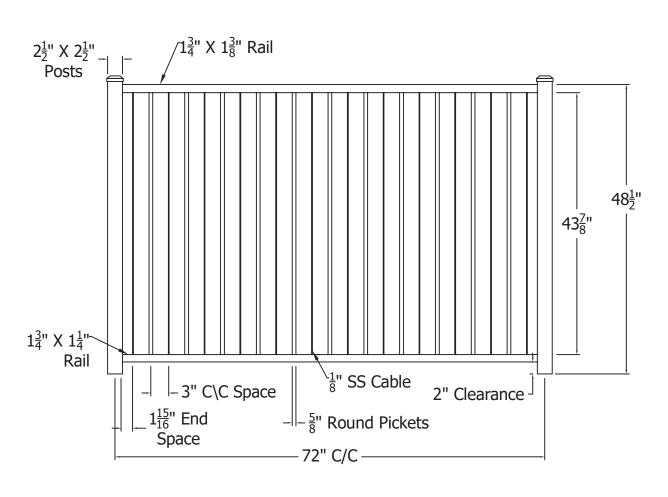
STYLE: DRAWN BY: EH DSI DATE DRAWN: **CF 220** 03-17-2020 SCALE = 1":1" AS SHOWN: 48<sup>1</sup>/<sub>2</sub>" T 3446 US 6 EAST LOC: Z:\Aluminum\Cable Bremen, IN 46506 DRAFT NO.: Fence\Updated Standard diggerspecialties.com 20200317-1E Drawings\Section
