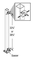
NOTE: For glass panels less than 30" wide or heights less than 32", insert glass into bottom rail, then fit top rail down over glass. Attach top rail to mounts.
